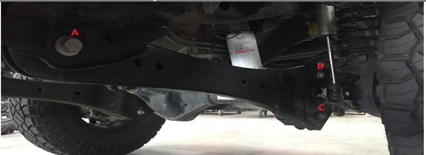
Figure 9: Radius Arm Bolt Locations
