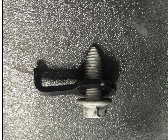
Figure 47: Bump Stop Spacer Orientation
