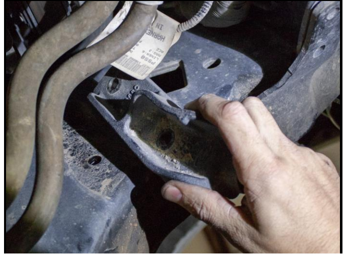
Figure 28: Stabilizer Bracket Removed
