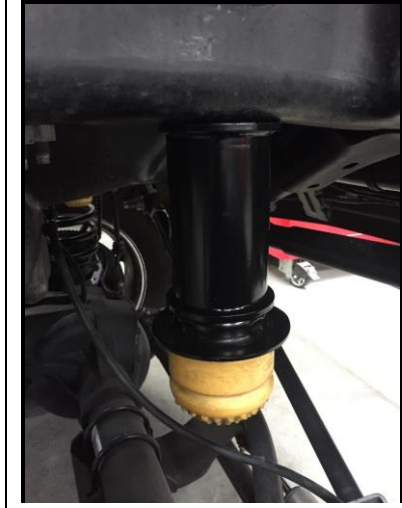
Figure 49: Bump Stop Spacer Assembled
