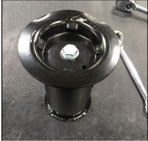
Figure 46: Bump Stop Spacer Assembled
