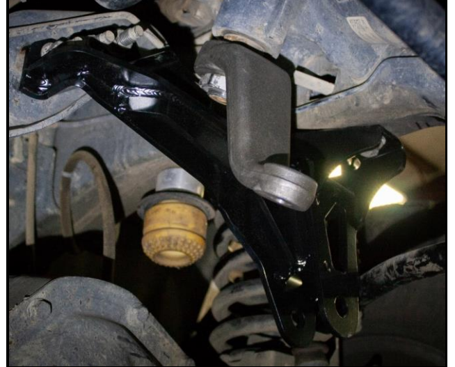
Figure 26: Cognito Track-Bar Bracket Installed
