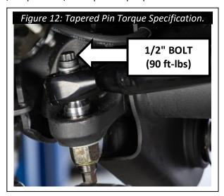
**10.** The following instructions are to adjust the steering wheel back on center. Make sure the vehicle is in park with the emergency brake activated, then start the engine. Loosen drag link adjuster sleeve and adjuster lock, slide the lock out of the way. Rotate the drag link adjuster in the appropriate direction to center the steering wheel.
