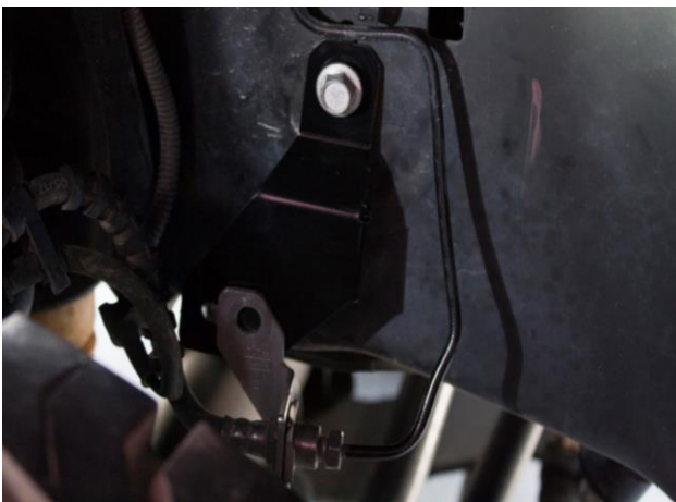
Figure 3: Passenger Brake Line Bracket
