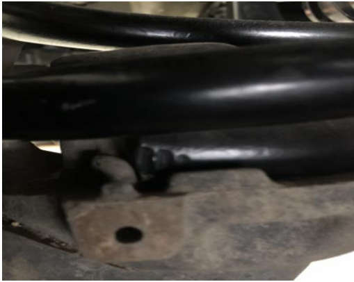
Figure 14B: Bottom Spring Pig-tail Orientation
