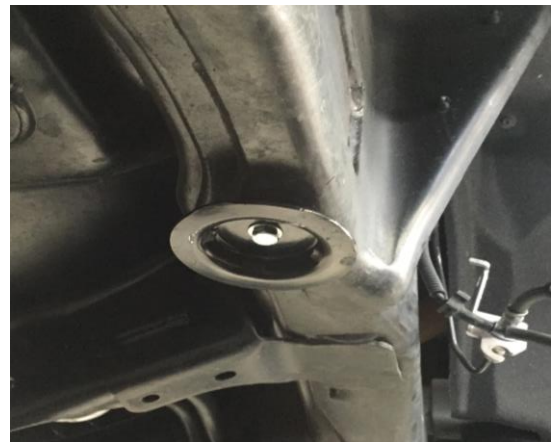
Figure 10B: FSD Bump Stop Spacer Hardware
