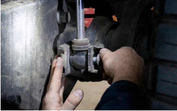
Figure 16A: Front Lower Shock Mount
