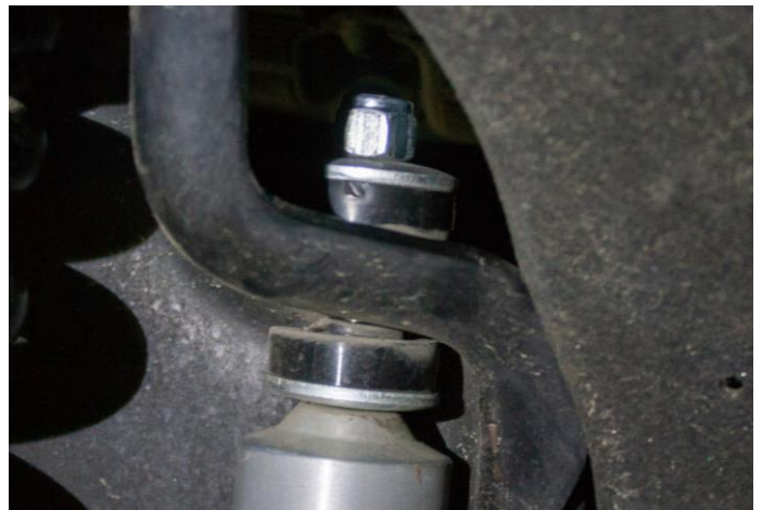
Figure 15B: Top Shock Mount Installed
