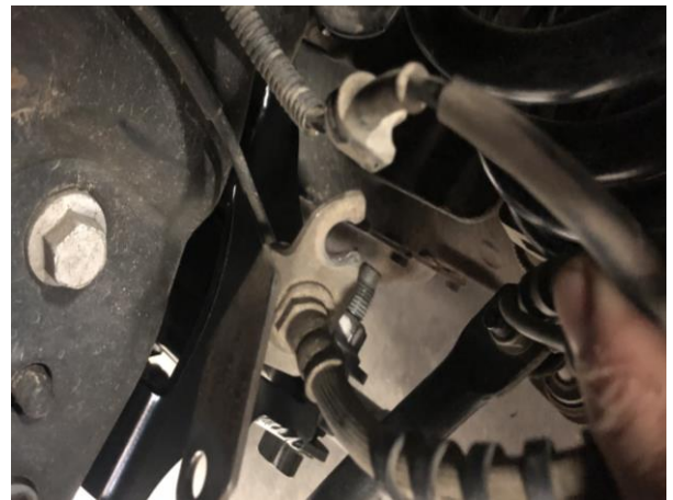
Figure 2B: Driver ABS Line Removal
