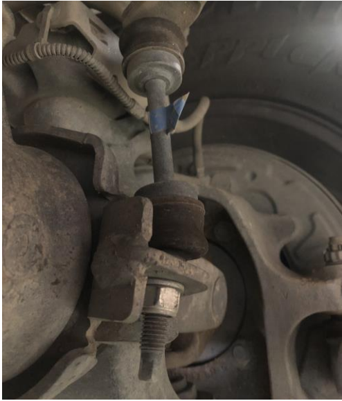
Figure 7A: OE Sway-Bar End Link
