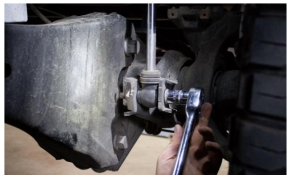
Figure 8B: Front Shock, Lower Mount
