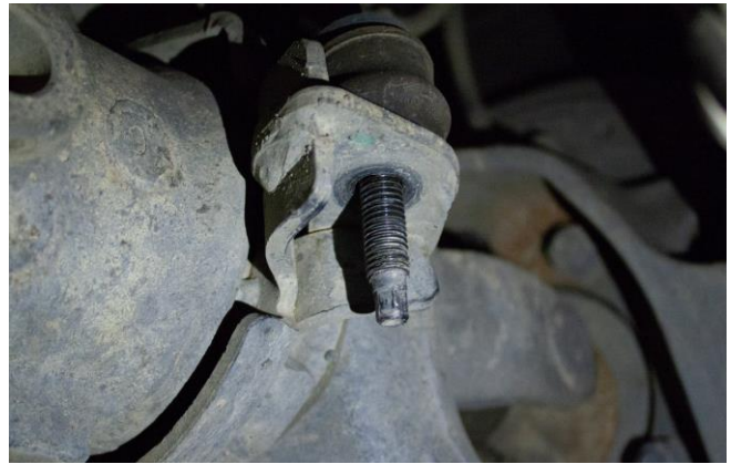
Figure 7B: OE Sway-Bar End Link, Nut Removed
