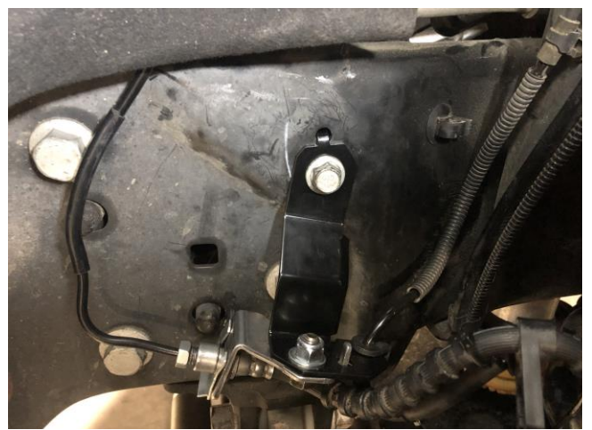
Figure 4: Driver Brake Line Bracket
