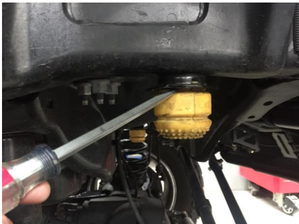
Figure 10A: OE Bump Stop Spacer
