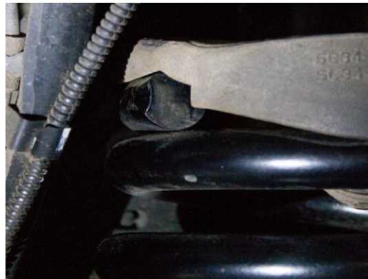
Figure 14A: Coil Spring and Isolator Orientation
