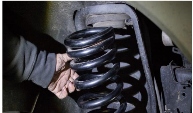
Figure 9B: Spring Removal
