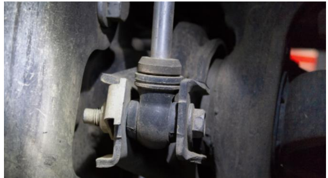
Figure 16B: Front Lower Shock Mount Installed
