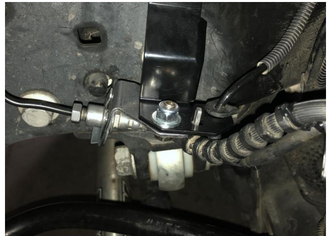
Figure 6: Passenger Side ABS Line Routing
