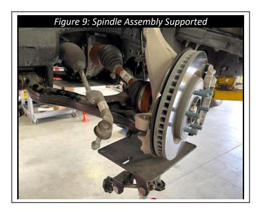
**11.** Remove the nut holding the UCA to the spindle and remove the UCA from the spindle. Ensure that the spindle does not fall over or put tension on the ABS sensor wire and the brake lines.
