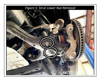
**7.** Remove the LCA pivot bolts. Swing the LCA downward and free of the strut. Place the hardware safely aside, it will be reused later.
