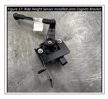
**20.** <u>Driver Side Only:</u> Install the ride height sensor back into the factory location using the factory hardware. Thread the ride height sensor linkage into the threaded hole located on the side of the Cognito UCA.
