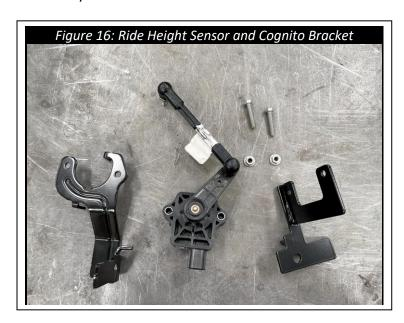
**19.** <u>Driver Side Only:</u> Attach the sensor to the Cognito ride height sensor bracket using the factory hardware. The arm on the sensor will be facing towards the front of the vehicle.
