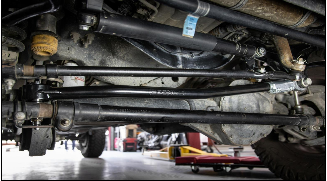
Figure 20: Installed Track Bar.
