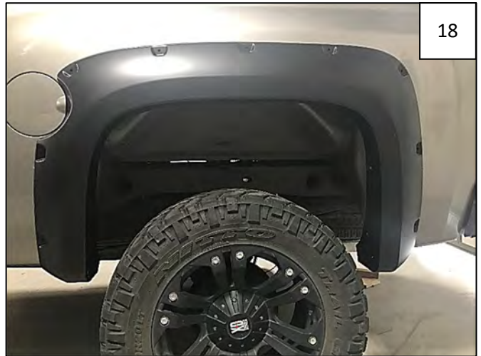
Apply pressure to outward face of the flare towards the center of the vehicle and tighten all screws.
