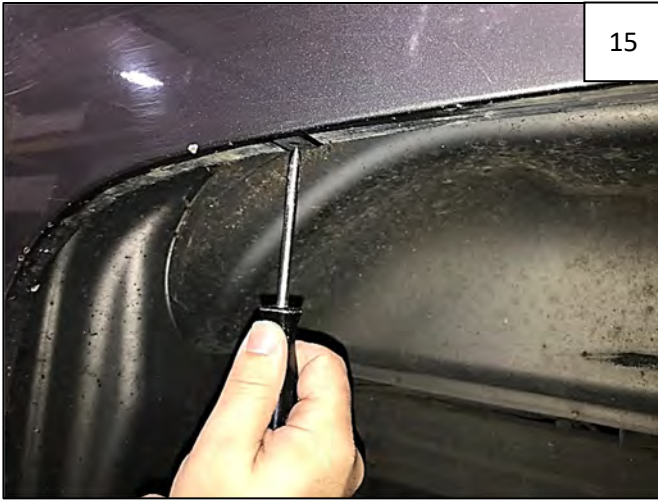
Use an awl to poke a hole through "U" Clip, Mounting Tab, and factory hole, for ease of screw installation.
