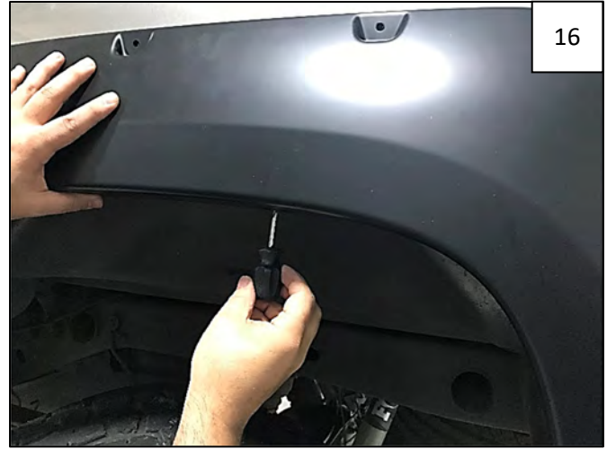
Reposition flare on fender and start a Long #10 Truss Head Screw through flare and into each "U" Clip installed in Step 14.
