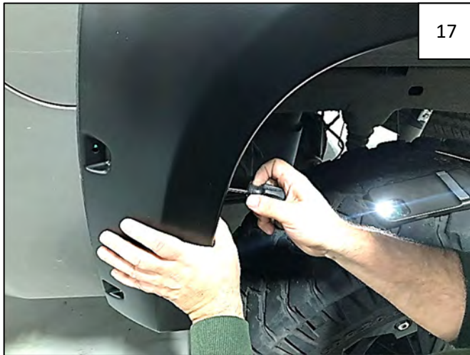
Start 4 Short #10 Truss Head Screws through flare and into "S" Spring Clips installed in Step 12. If needed, use an awl to line up holes.
