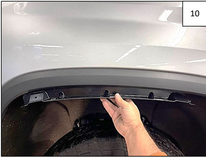
Install Inner Bracket using 2 T15 Torx screws retained in Step 9. Tighten both fasteners.
