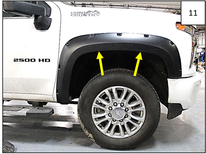
Align flare on vehicle and install 2 supplied Truss-Head Screws into clips on Inner Bracket as indicated by arrows.
