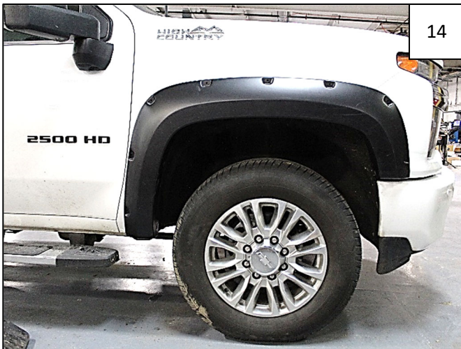
Complete Front Flare Installation.
