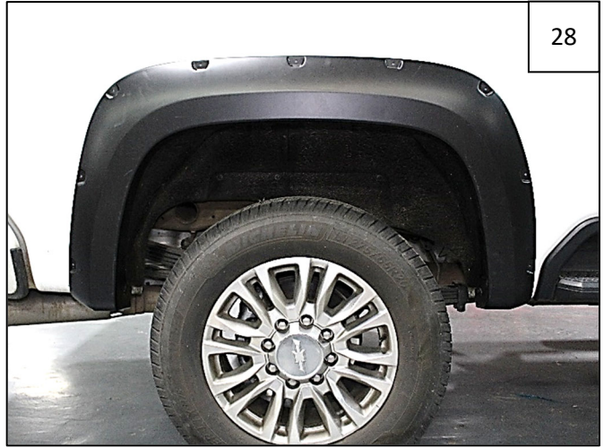
Completed Rear Flare installation.
