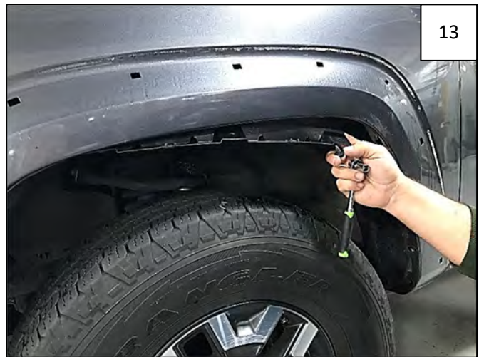
Line 3 holes in Inner Bracket with 3 uppermost holes in fender. Start 3 supplied 20mm Hex Screws through Inner Bracket and into holes in fender. Tighten screws.
