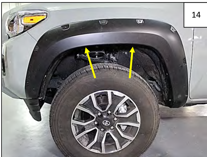
Aligning flare on fender and pressing toward vehicle, start 2 supplied 20mm Hex Screws through flare and into clips installed on Inner Bracket.
