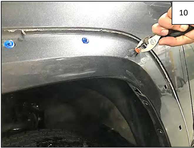
Use a vise grip or pliers to remove 1 factory clip as indicated by circle in Step 9, pulling with a rocking motion.
