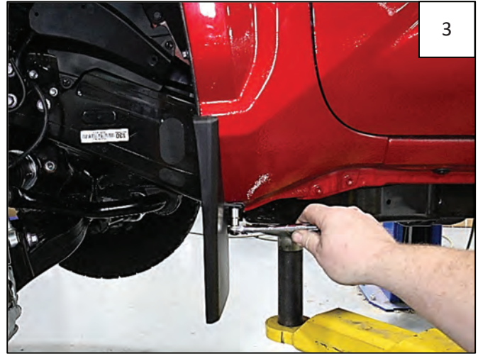
Remove 1 factory screw from underside of mudflap. Remove and discard mudflap.
