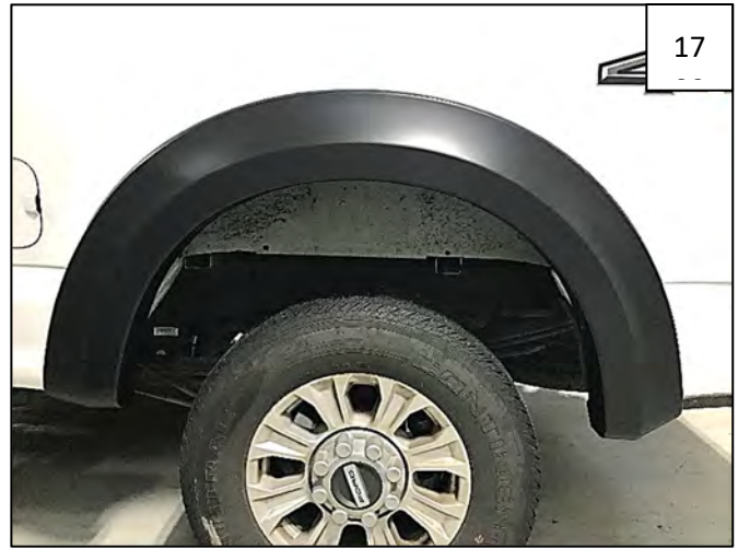
Completed Rear Flare Installation.
