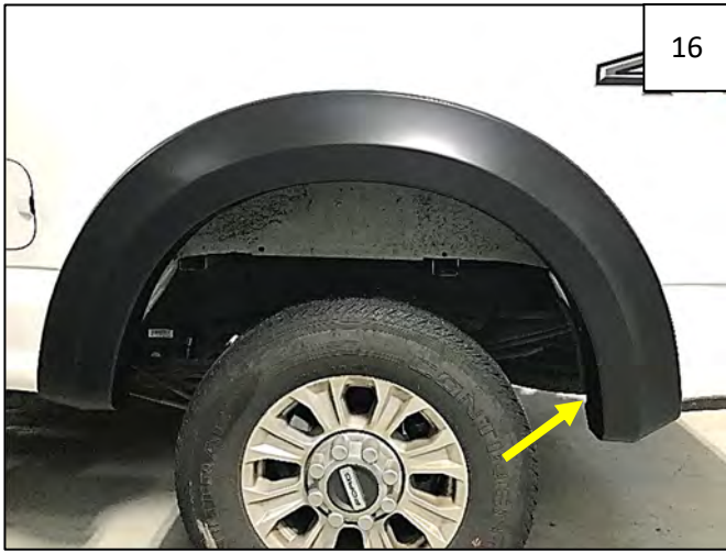
Install supplied Plastic Retainer through flare and into factory hole at rear of wheel well.
