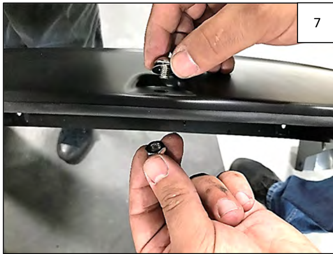
7 Place a supplied Pocket Nylock Nut over the end of each bolt and tighten using a 1/2" wrench for the Nut and the supplied T-45 Torx Bit for the Bolt. Repeat for all pockets.
