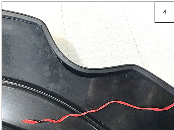
Correctly-installed edge trim around gas door.
