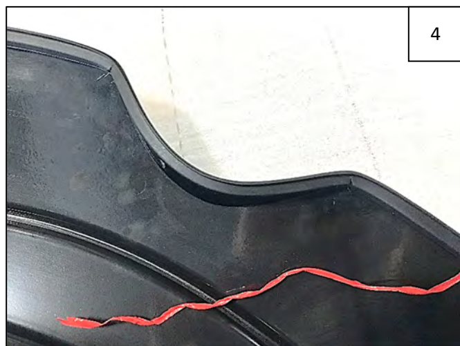
Correctly-installed edge trim around gas door.
