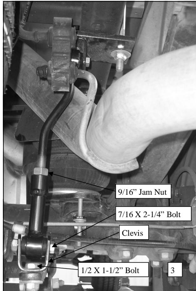
7. Assemble end links as shown in photos with 9/16" nut on the threaded half. Leave loose for adjustment. Insert hourglass bushing first and then sleeve into the loops of the end link assembly. **Lubricate the bushing and sleeve to ease assembly**
