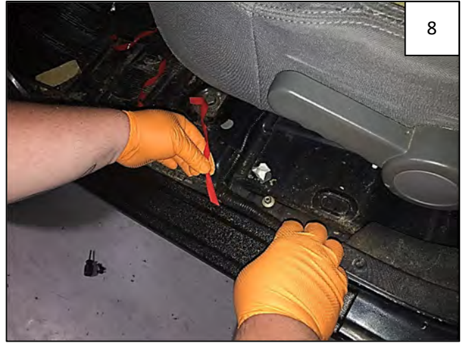
Repeat for other tape leader from door sill area as shown in Step 6. Do not peel tape from underside of part yet. Press part against vehicle in both sill areas.
