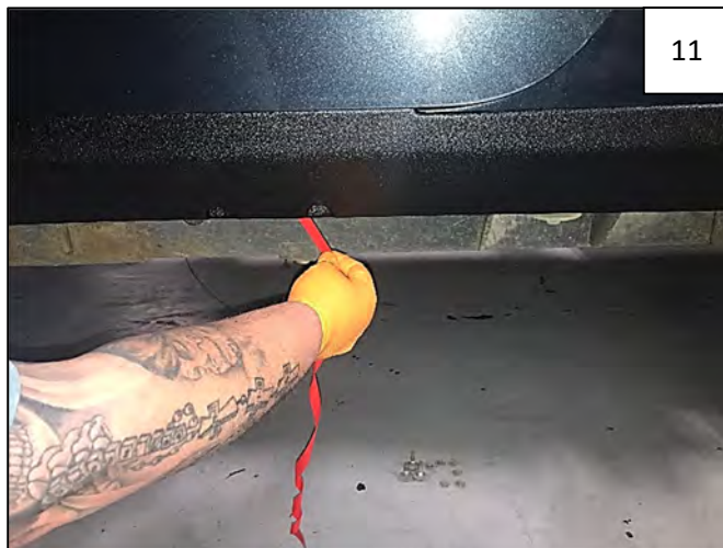
Starting with tape leader marked #1 in Step 10, carefully pull red tape leader at a 45 degree angle down and away from part to release from the tape, pressing against part as you go.
