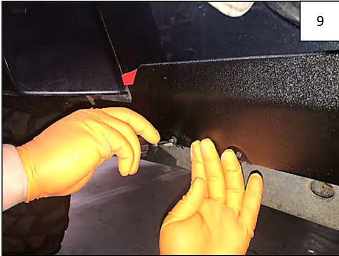
Remove 1 screw installed in Step 5.
