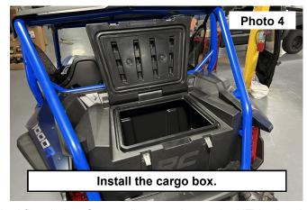
5. Aline the (4) holes in the bottom of the cargo box with the bed floor holes. Secure the cargo box to the UTV using the supplied hardware in each mounting hole. Install (1) Flat washer and (1) Button head bolt and tighten using a 4mm Allen Wrench. See Photos 5 and 6.
