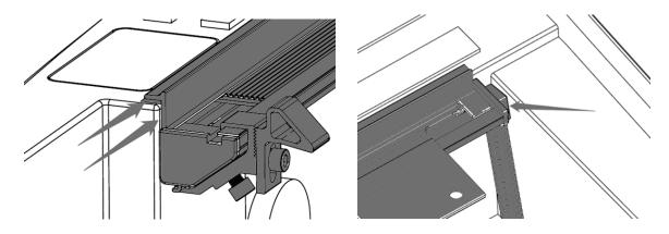
5. Place one clamp (F11) at the front of the side rail and one at the rear (please make sure the rear clamps is placed on the position that is closest to tailgate). Tighten the clamps each side. Then insert the drain tubes (F4) into the front of bed wall.
