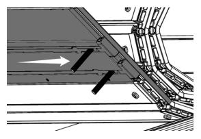
8. Close the cover front panel, and insert the Front Bolts (F6) into the 2 bolt holes of side rail mounting plate.
