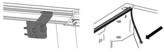
6. Place the hard roll up cover (F1) on the side rails.
