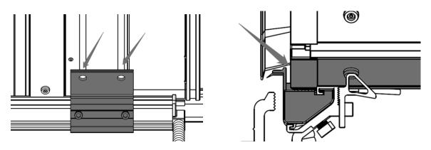
7. Roll up the cover front panel, making the back of front panel facing up. Insert the Front Bolt (F6) into the grooves of the front panel.
