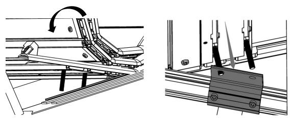
9. Insert the Security Straps (F5) onto the Front Bolt firstly, then insert Flat Washer (F7), Spring Washer (F8), and T Type Nut (F9). Tighten the T type nut firmly.
