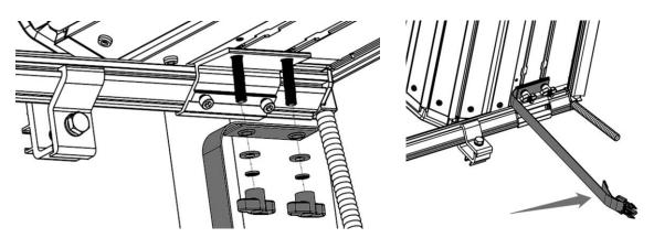
10. Close the cover, adjust the locking base back-and-forth to accommodate the groove of the rear panel. Try to close and open the cover rear panel several times. Make sure the Locking Base does not interfere with the groove of cover rear panel. Then tighten the bolt to fix the locking base on the side rail.
