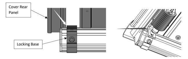
11. If the locking pin on the cover interfere with the locking tongue on the locking base, adjust the locking tongue up and down to a proper position, then tighten the bolt to fix the locking tongue.
