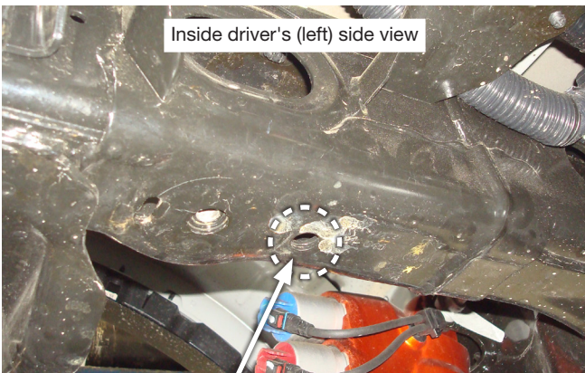
Index the socket-head cap screw into the hole forward of the jounce bumper mounting hole.
