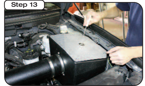
Step 13 Install the pre-oiled filter in the housing and tighten down clamp. With button head screws, install housing cover and tighten using 5/32" allen key.
