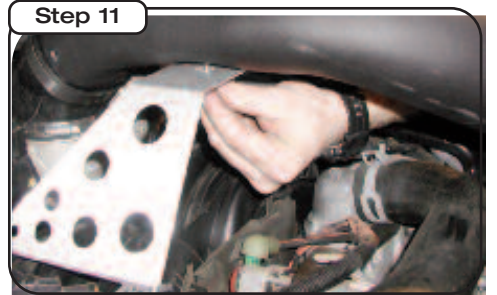
Step 11 Line up the mounting holes on the intake duct and tighten assembly with the provided screws and washers.
