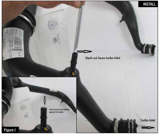
Refer to Figure I for Step 18 (For V6-3.5L (tt) only, not necessary on V6-2.7L (tt))
