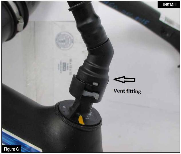
Refer to Figure G for Step 16 (For V6-3.5L (tt) only, not necessary on V6-2.7L (tt))
