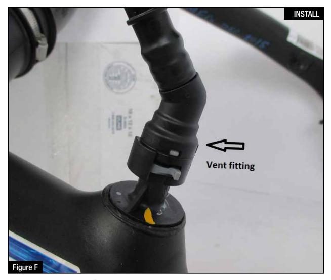
Refer to Figure F for Step 14. (For V6-3.5L (tt) only, not necessary on V6-2.7L (tt))
