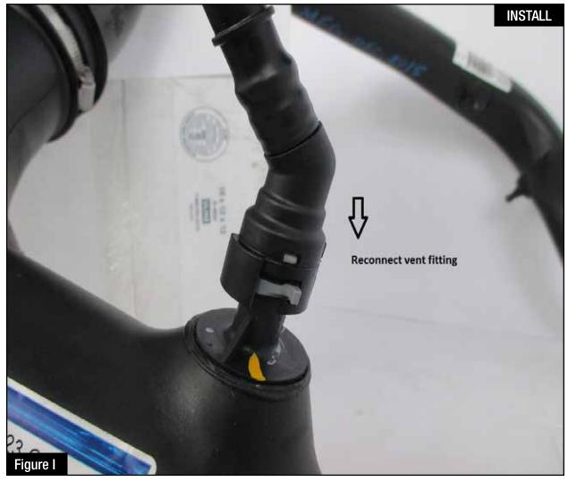
Refer to Figure I for Steps 17-18. (For V6-3.5L (tt) only, not necessary on V6-2.7L (tt) )
