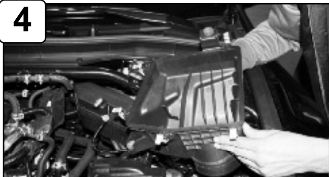
With 10mm socket or wrench loosen the bolt securing the bottom half of the air box and remove.
