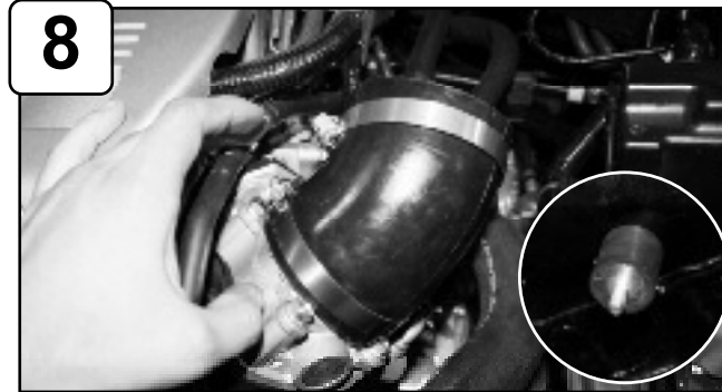
Install elbow coupler to throttle body and position using clamps provided. Do not tighten. Install isolation mount to threaded hole on inside of engine compartment.
