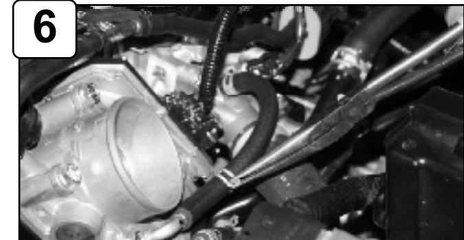
Replace throttle body coolant line with 5/16" hose provided and secure with clamps used from step 5.
