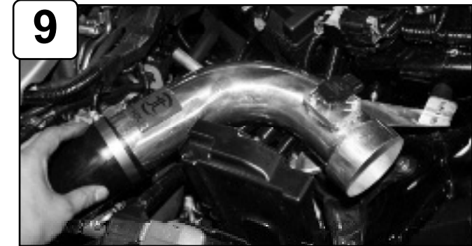
Install intake tube into vehicle and position tab to isolation mount and coupler.
