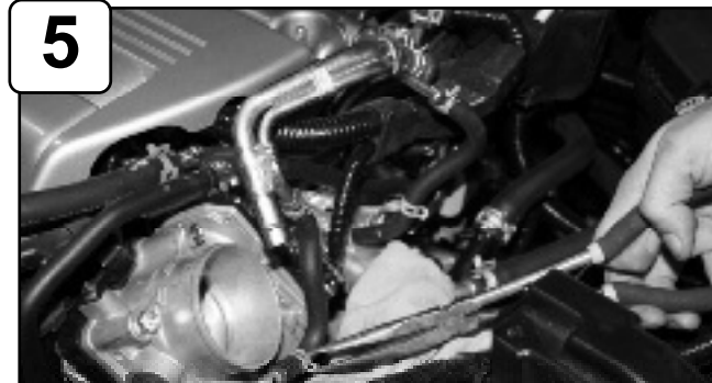
Remove crank case line attached with throttle body coolant line. Have a shop towel or rag handy to catch any leaking coolant. Use pliers to remove both lines. Save small clamps for later install. Caution: Coolant may leak from line when removing!
