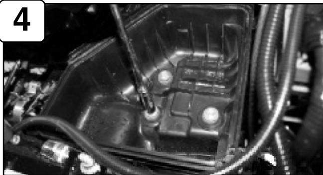
4 With 10mm socket or wrench loosen the 3 bolts holding in bottom half of air box and remove.
