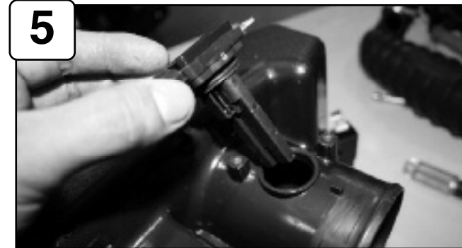
5 With phillips screwdriver loosen and remove MAF sensor.
