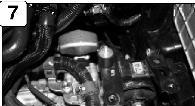
7 Install M6 isolation mount to air box bracket.
