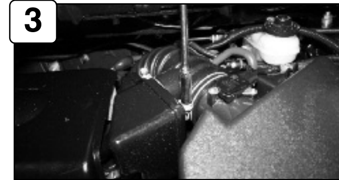
3 Disconnect MAF sensor and loosen clamp using 10mm socket or wrench. Unclip upper half of air box and remove. Loosen clamp with pliers on throttle body and remove stock intake tube.
