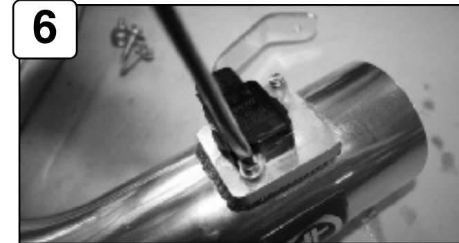
6 Install MAF sensor to upper intake tube assembly and secure using provided M4 screws.
