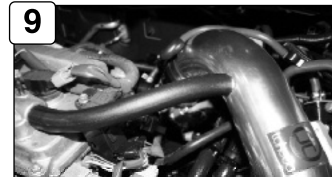
9 Remove engine cover using 10mm socket or wrench. Remove stock crank case line and replace with provided 5/8" hose. Re-install engine cover and tighten.
