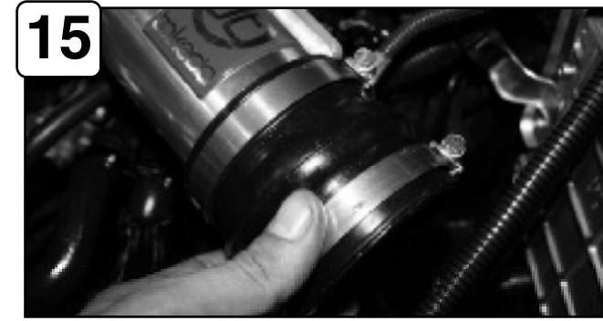
15 Attach hump coupler with clamps to upper intake tube assembly. Do not tighten.
