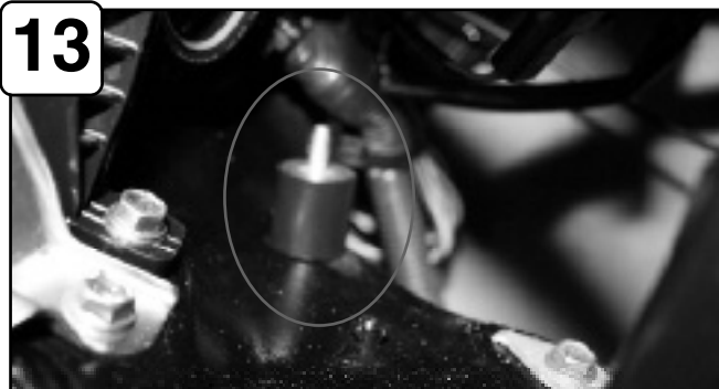
13 Install and tighten isolation mount to frame.
