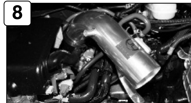
8 Install upper intake tube assembly into vehicle with provided reducer coupling and clamps. Do not tighten.
