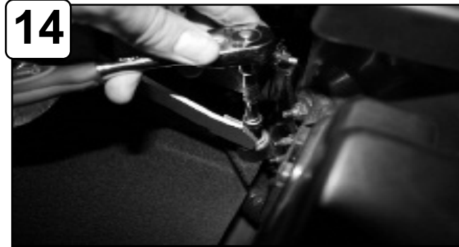
14 Tighten intake bracket using provided flat washer, wavy washer and nut.
