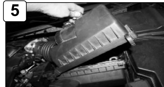
Remove upper half of air box and stock tube w/ carbon attachment assembly.
