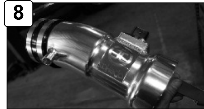
With provided M4 screws, install MAF sensor to new intake tube. Attach coupler to tube with clamps provided. Do not tighten.
