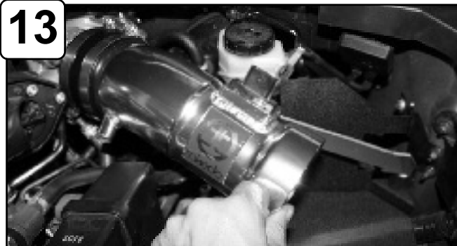
13 Install intake tube assembly and position tab to isolation mount. Do not tighten.
