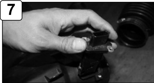
Remove MAF sensor using phillips screwdriver.
