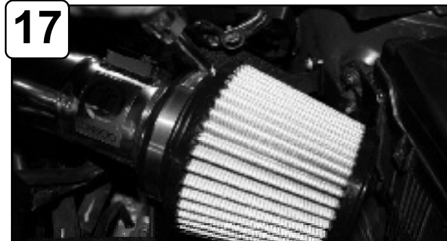
17 Install air filter and tighten using 5/16" nut driver. Re-connect battery terminals.
