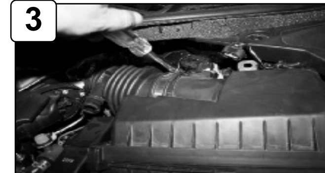
With 5/16" nut driver loosen clamps on stock intake.
