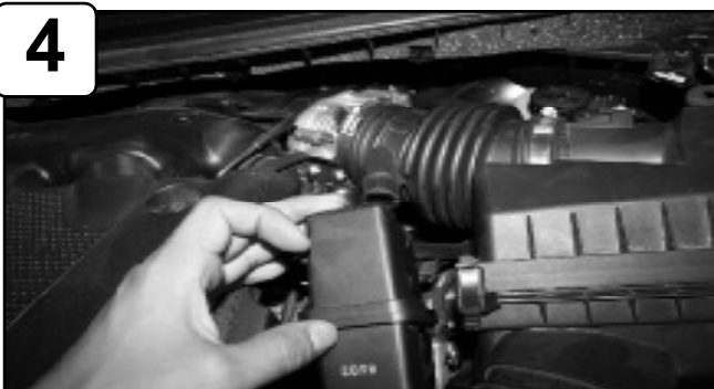
With 5/16" socket or wrench loosen crank case line. Disconnect MAF sensor harness.
