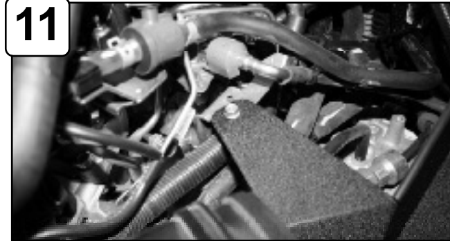
11 Install housing into vehicle and position. Re-secure tab on housing with bolt from step 10.
