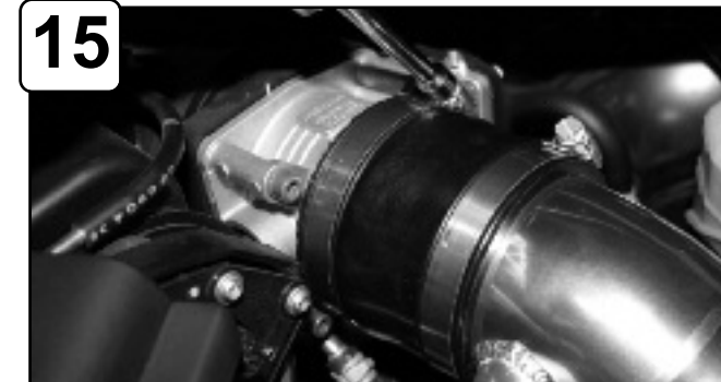
15 Tighten all clamps using 5/16" nut driver.
