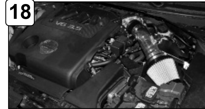
18 The installation of your Takeda performance intake is now complete. Place the included CARB EO sticker on or near the intake system on a smooth, clean surface. E.O. identification label is required in passing the smog check inspection.
