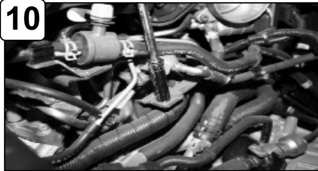
10 With 10mm socket or wrench loosen bolt on engine.
