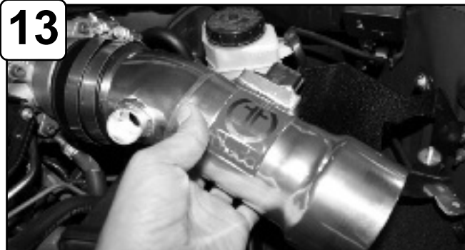
13 Install intake assembly and position tab to isolation mount. Do not tighten.
