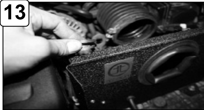
13 Remove OE grommets from air box and install to hole cut outs on top of housing.
