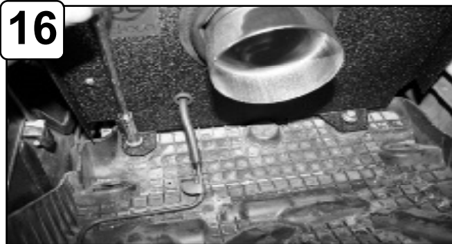
16 Tighten screws using 10mm socket or wrench.
