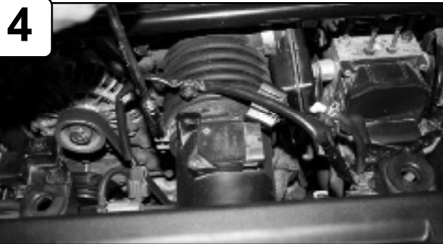
With 10mm socket or wrench loosen clamp holding in air box.
