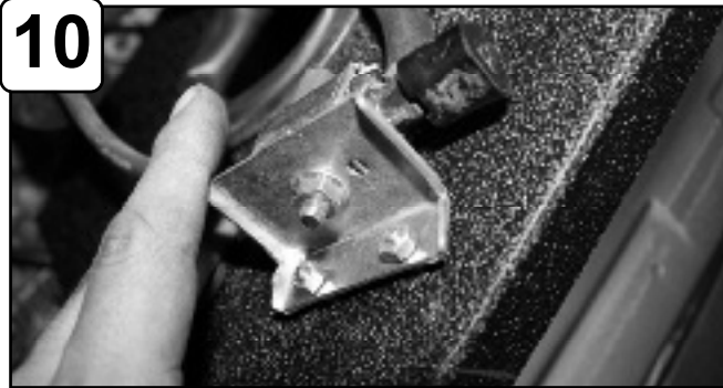
10 Attach VSV sensor to back of housing and secure using provided M4 screws and nuts.
