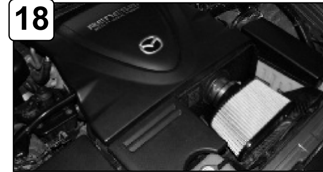
18 The installation of your Takeda performance intake is now complete. Please check all components and re-tighten if necessary. Thank you for choosing Takeda! Place the included CARB EO sticker on or near the device on a smooth, clean surface. E.O. identification label is required in passing the smog check inspection.
