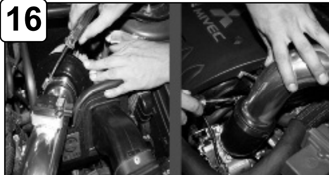
Install filter and tighten using 5/16" nut driver. Tighten all remaining clamps using 5/16" nut driver.
