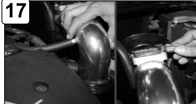
Install provided 5/8" hose to engine and tube. Reconnect MAF sensor harness. Reconnect battery terminals.
