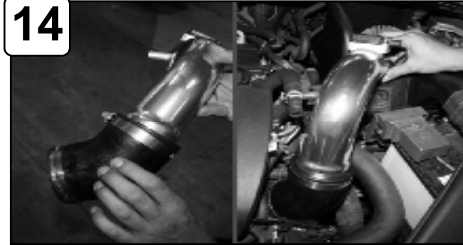
Attach elbow coupling with clamps to tube. Position tube to throttle body and tab on tube to isolation mount.
