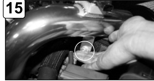
With M6 nut, wavy and flat washer provided, secure tab and tighten using 10mm socket or wrench.
