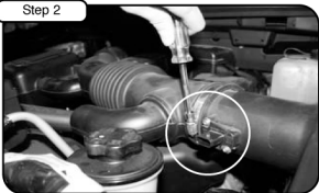
Disconnect the MAF sensor harness. Loosen the clamp on the airbox tube using a 5/16" nut driver.
