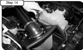
Position tube and tighten all clamps using 5/16" nut driver. Re-connect MAF sensor harness.
