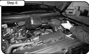
Remove the stock intake tube from the vehicle.
