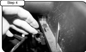
Disengage the 3 clips which secure the upper portion of the airbox. Remove the center clip which is not used with the aFe intake.
