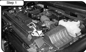
Complete Stock Intake. Disconnect the battery.
