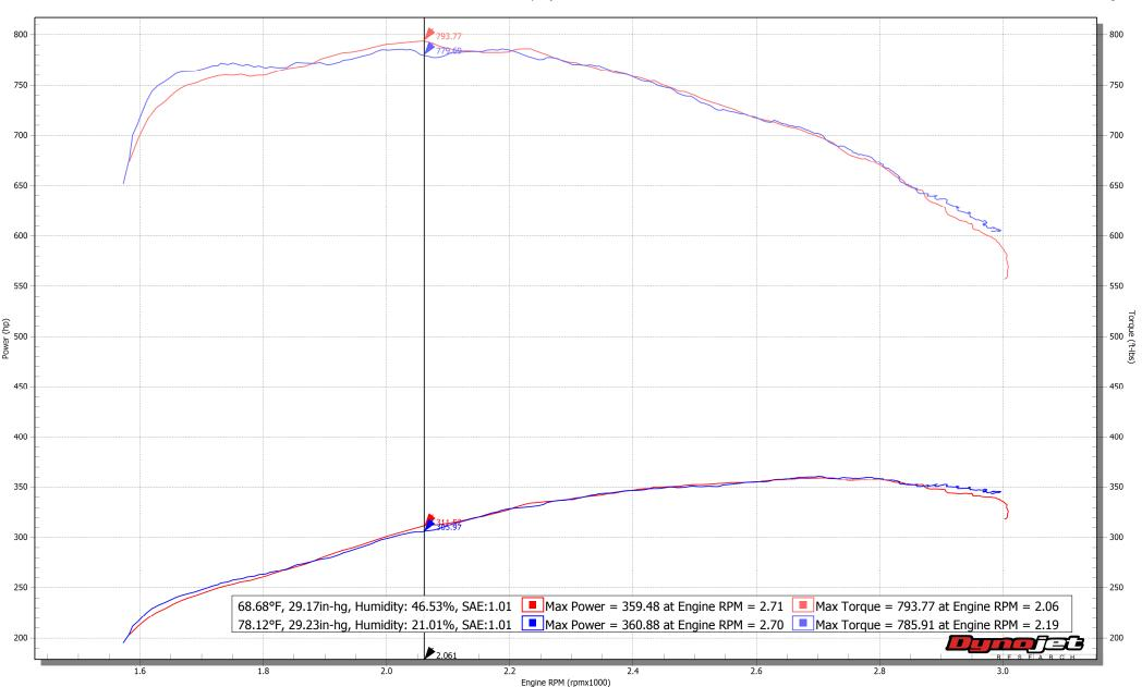
Dodge Ram 2500 6.7L (td) 2016\_53-10007D\_6.wp8 [ At: 3:17:39 PM, Monday, June 18, 2018 ] [ As tested on Dynojet Model 424xLC Linx ] [ CF: SAE 1.01 ] [ RPM: OBD2 ] [ Linx not connected ] [Title: Quantum 53-10002D] Notes: 53-10002D AIS, OEM Exhaust, OEM Intercooler, 4th Gear, 40% Load, LT285/75-18
