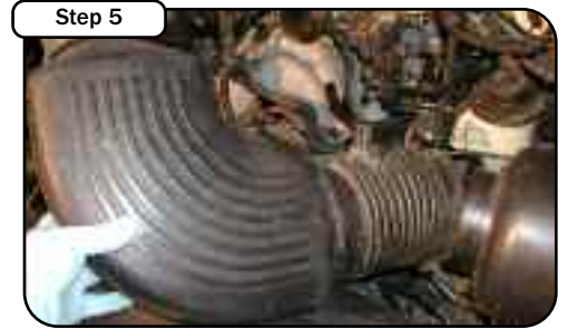
Unplug the IAT sensor and remove the intake duct from the engine. On some 04-05 models the IAT sensor is not present.
