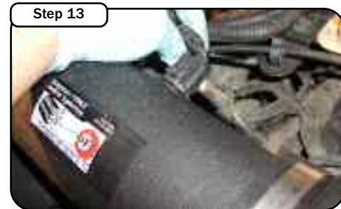
Install the rubber grommet into the IAT sensor location. Reinstall the IAT sensor and reconnect harness. At this time plug the MAF sensor into the harness and secure harness on the side of the housing with the included mounting holes. If you do not have a IAT sensor use the provided grommet and cap to seal the opening.
