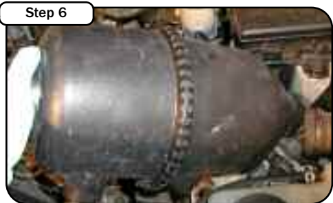
Lift air filter housing by pulling straight up it is held in place with 2 rubber gromets. On the back side of the canister is the MAF harness. Unplug harness from vehicle and remove.
