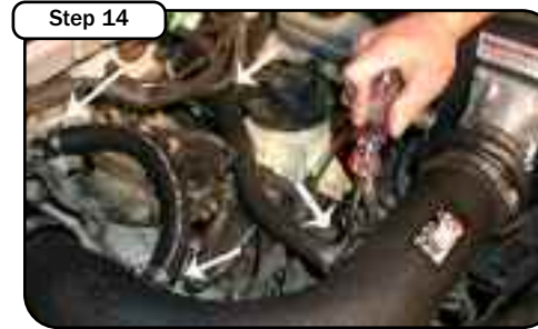
Install the 3/4" idle air bypass hose and the 5/8" breather hose on the intake tube and tighten down clamps. If you do not have a idle air bypass valve seal with the provided 3/4" vacuum cap. Install air filter and tighten down the clamp.
