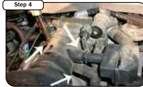
Loosen the factory hose clamp on the throttle body, and the 3/4" idle air bypass hose and the 5/8" breather hose. On some 04-05 models the IAB is not present.
