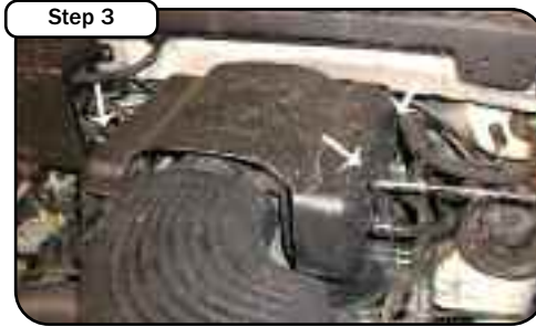
Remove the three 10mm bolts holding the throttle body cover.
