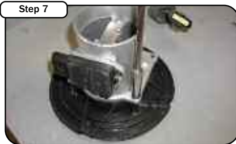
Separate the filter canister by unfastening the band clamp and removing the air filter. Disconnect the harness from the MAF sensor. Unbolt the MAF Sensor from the filter base and the short wire harness set aside for later use.
