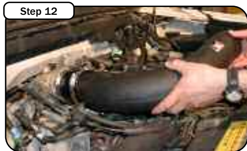
Install the smaller end of the intake tube into the throttle body coupler and insert other end into the hump coupler on the housing. Tighten down clamps on both couplers.
