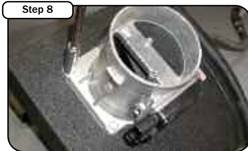
Mount the MAF sensor and MAF sensor gasket to the outside of the air filter housing. Use the (4) M6x1x20 screws and tighten down with a 10mm wrench.
