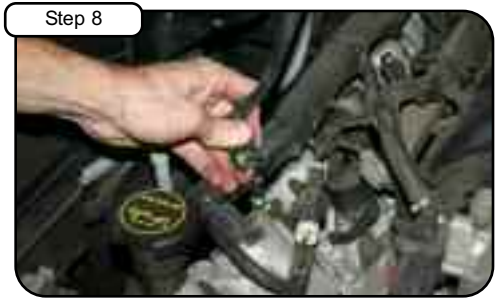
Remove factory crank case line from engine.
