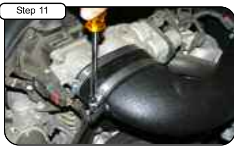
Tighten clamps with 5/16" nut driver.
