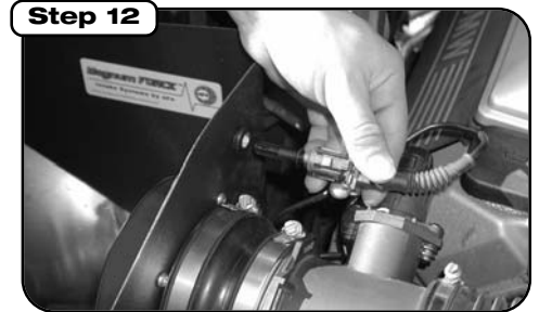
Install temperature sensor.
