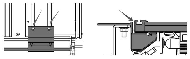
8. Roll up the cover front panel, making the back of front panel facing up. Insert the Front Bolt (F6) into the grooves of the front panel.
