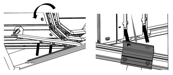
10. Insert the Security Straps (F5) onto the Front Bolt firstly, then insert Flat Washer (F7), Spring Washer (F8), and T Type Nut (F9). Tighten the T type nut firmly.
