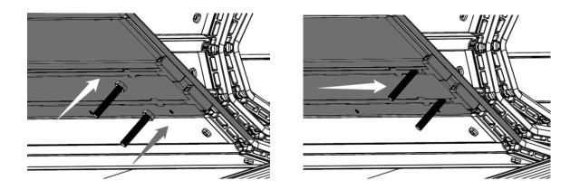
9. Close the cover front panel, and insert the Front Bolts (F6) into the 2 bolt holes of side rail mounting plate.
