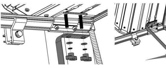
11. Close the cover, adjust the locking base back-and-forth to accommodate the groove of the rear panel. Try to close and open the cover rear panel several times. Make sure the Locking Base does not interfere with the groove of cover rear panel. Then tighten the bolt to fix the locking base on the side rail.
