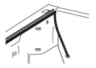
7. Place the hard roll up cover (F1) on the side rails.
