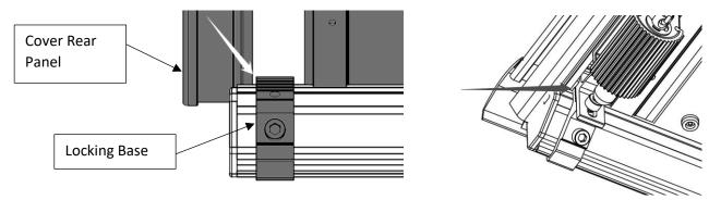
12. If the locking pin on the cover interfere with the locking tongue on the locking base, adjust the locking tongue up and down to a proper position, then tighten the bolt to fix the locking tongue.
