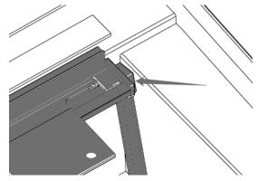
5. Place one clamp at the front of the side rail and one at the rear (please make sure the rear clamps is placed on the position that is closest to tailgate). Tighten the clamps each side.
