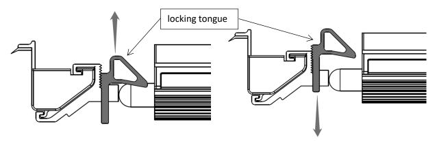
13. After truck tailgate closed, if the tailgate is not touching the cover rear panel rubber seal, there could be some water leaking on the tailgate part. Can adjust the whole cover a little closer to tailgate, by moving the side rail (F2/F3) a little back toward tailgate (loosen the side rail clamps to move, then tighten)
