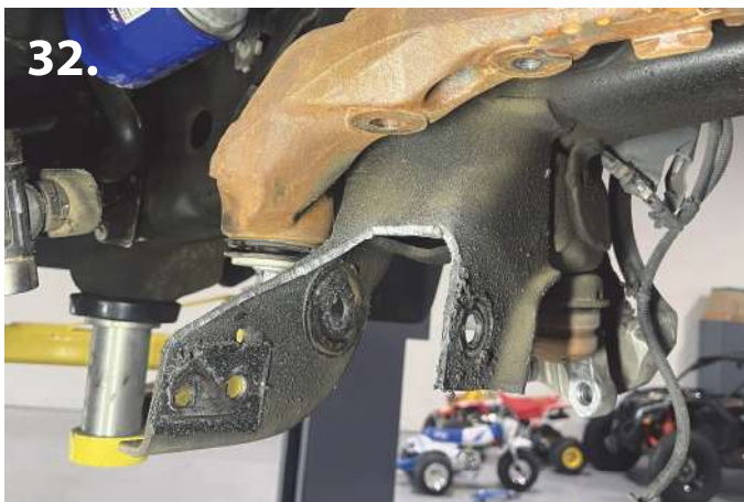
34. Remove cut piece and template (pics 32-33).
