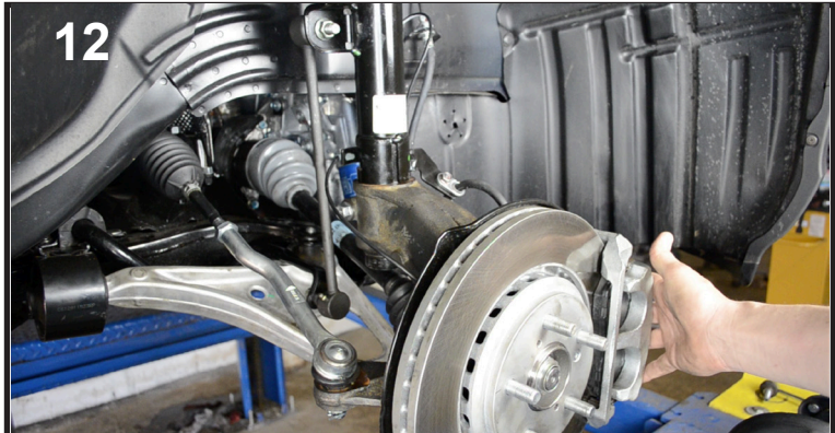
Install brake caliper. Install tie rod, ball joint, speed sensor wire, and axel nut. This is a reversal of the removal process.
