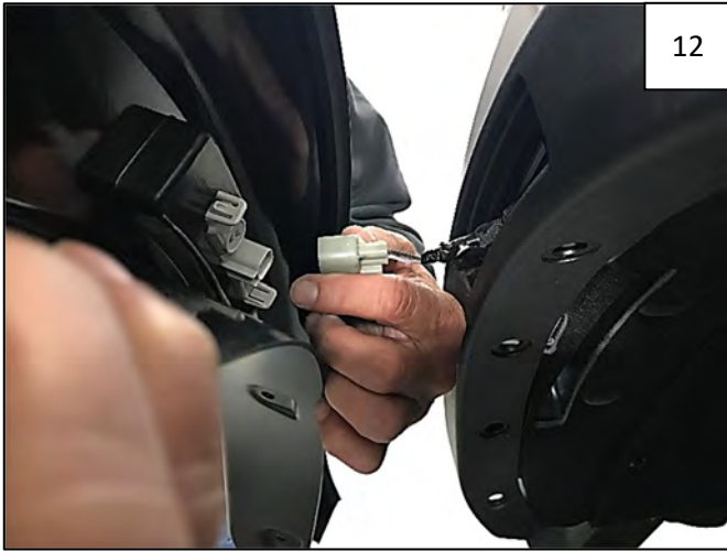
Hold flare on fender (it fits over factory flare) and reconnect the bulb/wire harness to the marker light.
