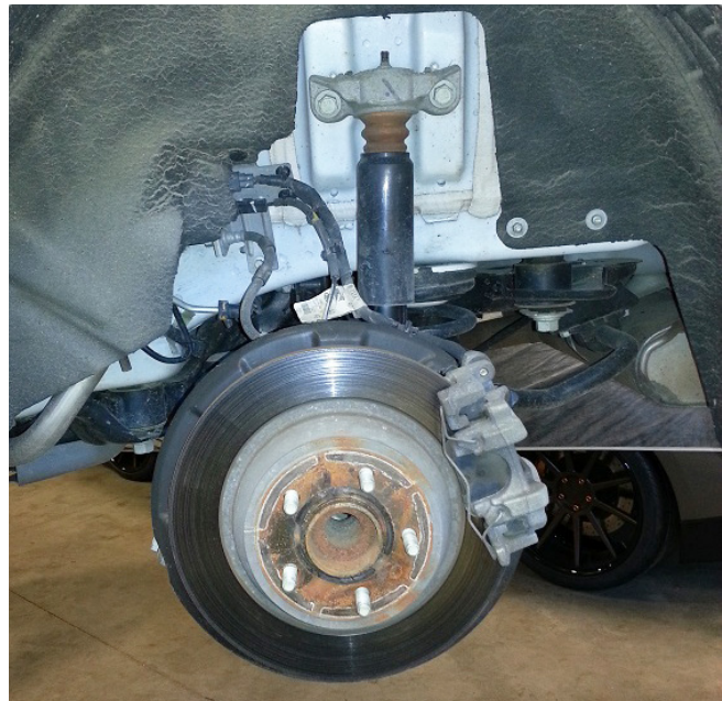
View of the rear wheel removed
