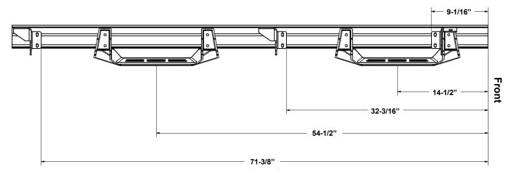
Loosely install the 8mm x 25mm bolts and flange nuts in the step and slide the step onto the rail.
